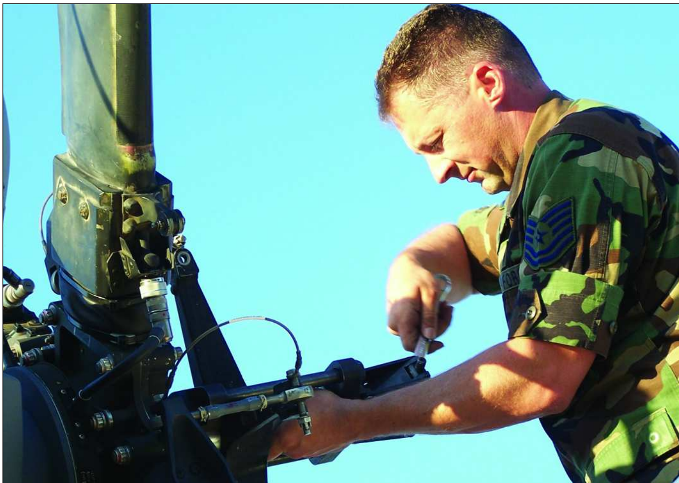
TSgt. Dan Starner, helicopter maintenance journeyman, 943rd Rescue Group, works on the tail rotor pitch beam after arriving in Portland, Ore.
