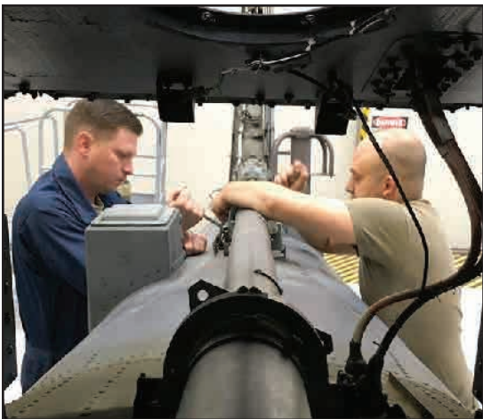
Top left: Tech. Sgt. Brandon and Staff Sgt. Michael, 943d Maintenance Crew Chiefs, install a Tail Rotor Drive Shaft during the assembly stage of the helicopter’s 600-hour phase inspection, March 19.
