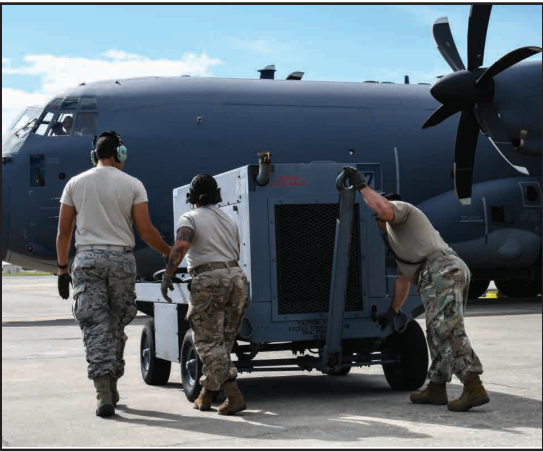
Bottom: 720th Aircraft Maintenance Airmen push a power cart closer to an HC-130J aircraft to hook up external power.
